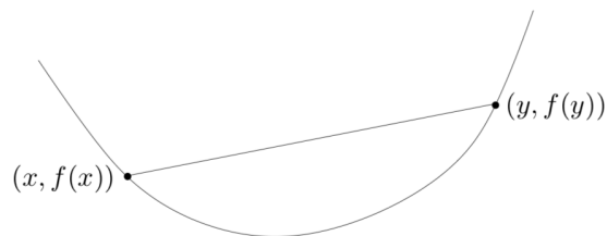
Figure 4.3: Graph of a convex function. The line segment between any two points on the graph lies above the graph.
